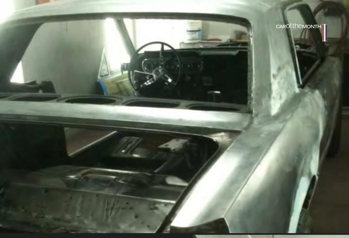
Knutson, and Dave Agnew) ended up doing a full restoration: Removing 11 layers of paint and Bondo, new cowl, new driver's side quarter, new door skins, new hood, new exterior everything - even down to the exhaust tips (custom made by a friend of mine). I splurged on the billet rear taillight housings and gas cap...because they just HAD to match his billet grills (he has two).
