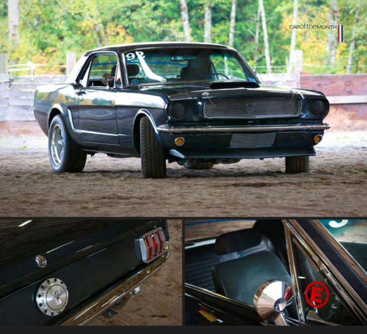
G-Force Comp 2 tires (225 front, 245 rear). A tach was added, as were 3 point seat belts, fire extinguisher, Fox front seats, Wilwood rear disc brakes, chin spoiler, and TCP complete subframe system. I got tired of taping up his headlights for track use, so I removed them altogether.
